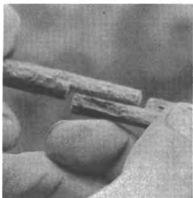
Left: Hand drill spliced to receive a softer tip (here yucca). Below: Splice wrapped with sinew, showing how to hide loose ends. Just pull the right-hand string and the noose will pull tight. Bottom: Spliced tip ready for service.
