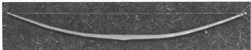
The bow, before final heating and finishing, draws 50 lb. at 15 1/4".
